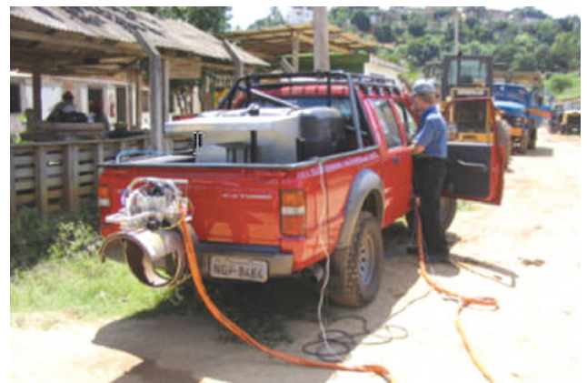
Figure 8. Scanner mounted on the cal block
