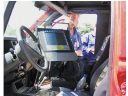
Figure 6. AGR Technology Design Focus-Scan phased array instrument mounted in the vehicle
