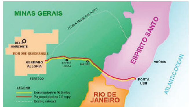
Figure 1. Route of iron ore slurry pipeline from the mine site to the shipping port
